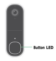
The Indicator LED is on the outside of your doorbell and indicates how the doorbell is operating. This section describes how the Indicator LED works if you didn't change the default LED settings. For information about changing the Indicator LED behavior, see *Control the doorbell button LED on page 23*.
