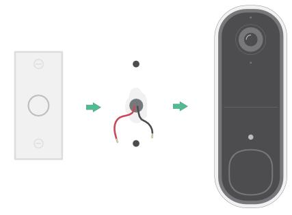
The equipment is intended to be supplied by approved external power source or ITE product (UL listed/ IEC 62368-1/ IEC 60950-1), whose output is complied with ES1/SELV/PS2/LPS, output rating 8-24Vac, minimum 0.65A, 50/60Hz, ambient temperature 45°C minimum.
