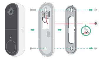
Place the doorbell on the mounting plate in a down-and-in motion.
