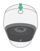
**Press and hold the pairing button for 3 seconds.** The camera wakes and the LED flashes blue for two minutes. Follow the instructions in the Arlo Secure App to add your camera to your Arlo account.
