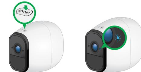
The camera LED blinks blue. When the camera is synced to the base station, the camera LED blinks rapidly to confirm sync.
