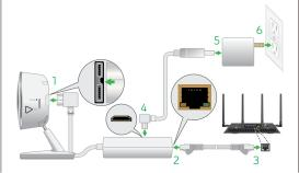
Power over Ethernet (PoE). Connect the Arlo Q Plus camera to a PoE switch using the included PoE adapter if you want to power and connect the camera to the Internet with a single cable.
