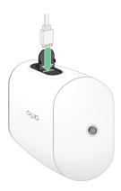
3. Connect the other end of the charging cable to a USB charging source such as a USB charging port or an AC power adapter.
